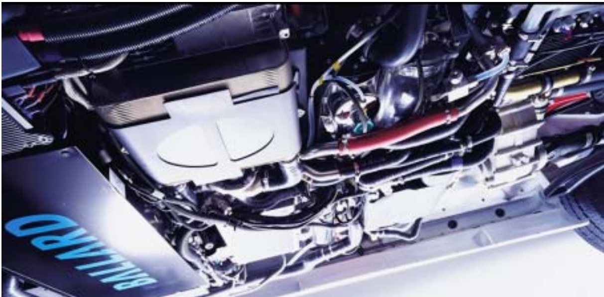
Figure 13: Fuel cell system in the floor of the Sprinter
