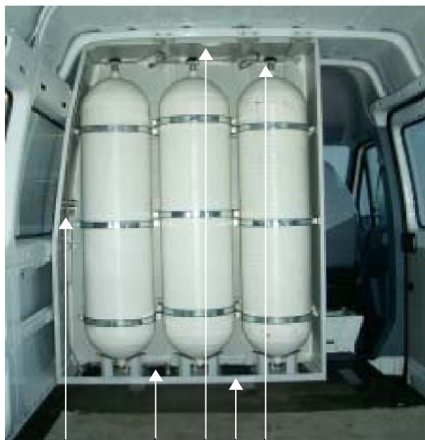
200 bar pressure gauge Ventilation Valves and piping
