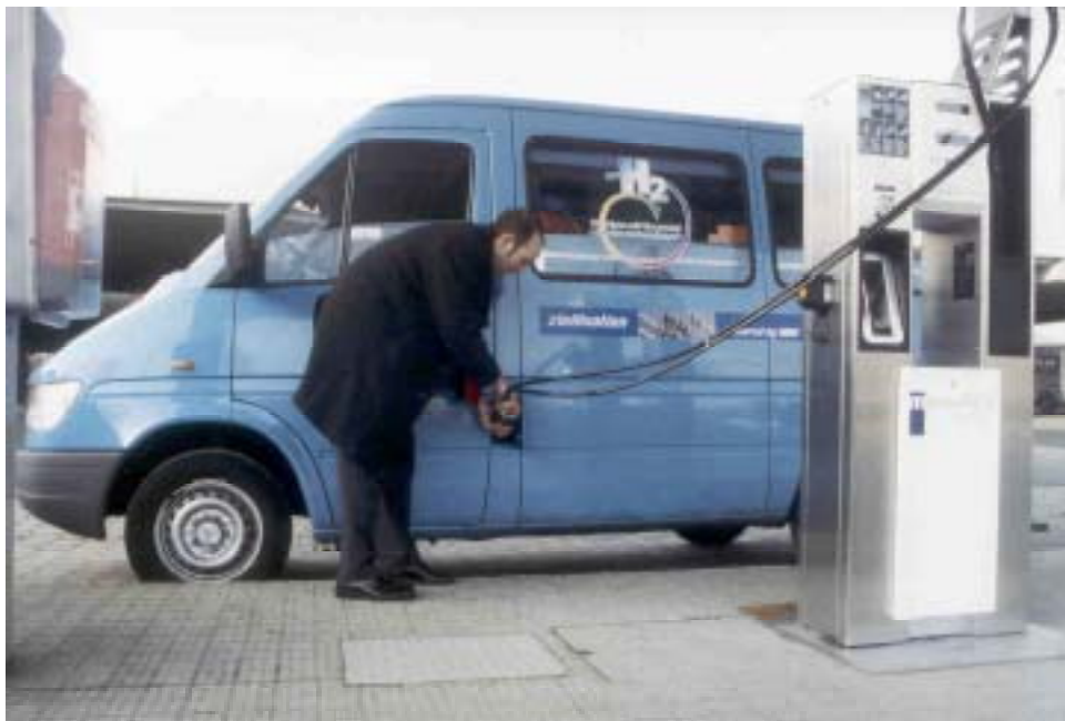
Figure 4: Van at the hydrogen refueling station
